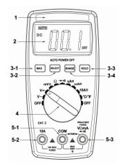
3.3.HOLD (Data Hold): Press the button, the reading is locked, press the button again, the lock is cleared.
